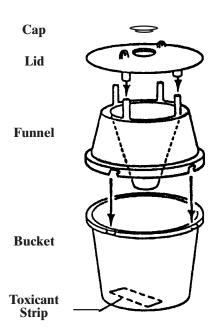
Join the bucket segment to the lid assembly by twistlocking the pieces together.
